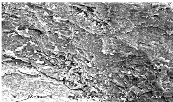
Fig. 3: SEM of CSH gel prepared using pretreated rice husk.
