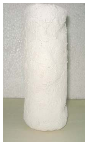
Fig. 5: Dried white gel prepared from CaO and amorphous silica (Ca/Si=2).
